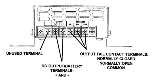
If wiring to a battery, the ungrounded battery connection must be fused.
