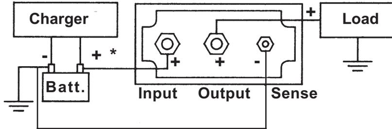
*\* It is recommended to provide over-current fuse or circuit breaker protection on the ungrounded connection as close to the battery as possible.*
